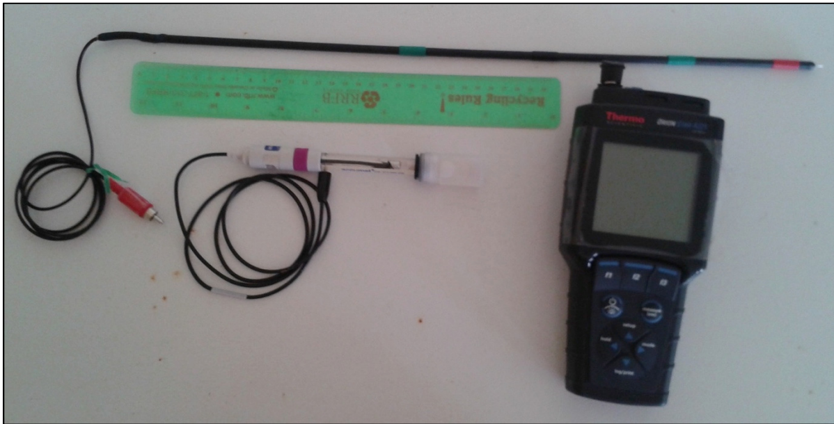
Figure 11 Constructed platinum electrodes (probes: top), accumet calomel reference electrode (bottom) and Thermo Scientific Orion Star A221 Millivolt Meter. Photograph taken by C. Skinner 2013.
